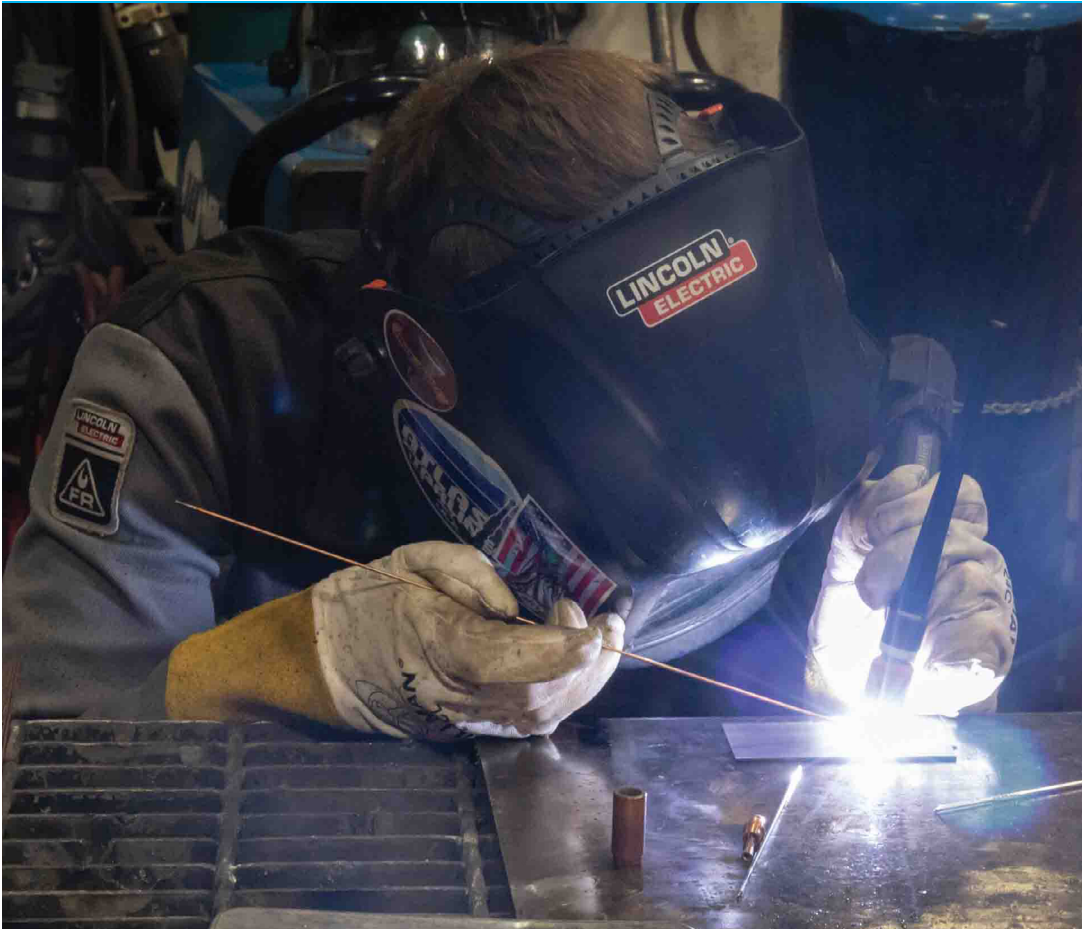
Alex Pazkowski demonstrates tungsten inert gas welding technique to students. Pazkowski teaches Shielded Metal Arc Welding (SMAW) where the class uses steels and consumables provided by companies in Michigan.
