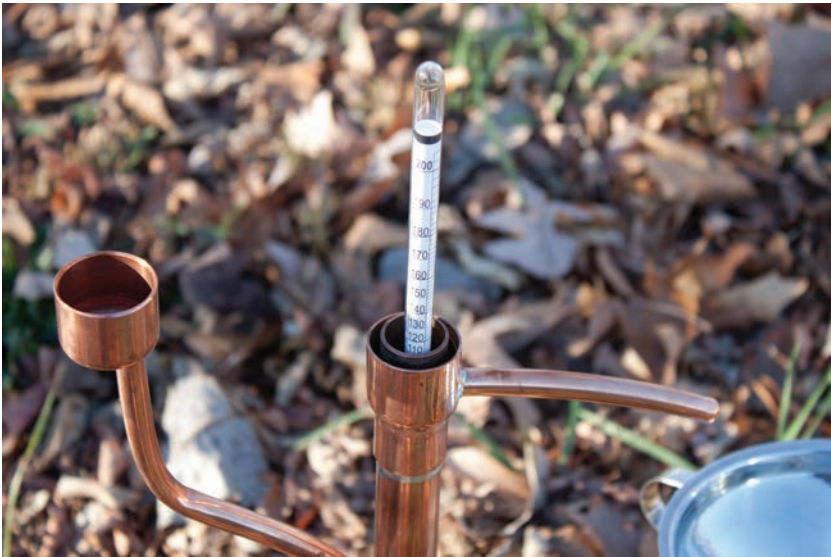
The large still is a five-gallon keg, also known as a compound still (compounding a reflux and a fractionating still). The copper 5-shaped section next to it (the one with the close up photo of the top of it) is known as a distiller’s parrot. The parrot measures the proof of alcohol exiting from the still.
